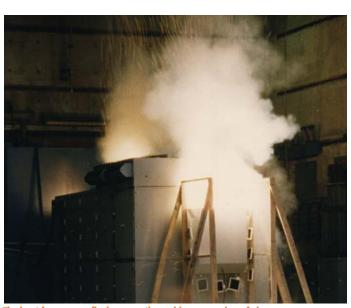
The heat from an arc flash causes the sudden expansion of air
